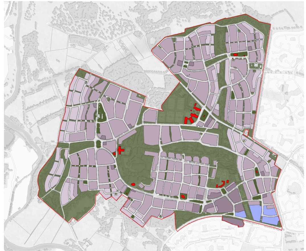
Figure 14: Grandhome's Regulating Plan, indicating the distribution of Transect Zones T3,T4,T5 and SD. Civic buildings are identified in red.
